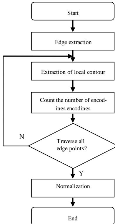
Fig. 2. Flow chart of LCDF feature extraction
